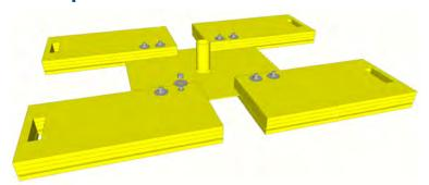
Fasten large flange washers and nuts on top of all plates with the washers contacting the plates first.
