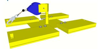
Install swivel top and SRL making sure to install all hitch pins with cotter pins installed.
